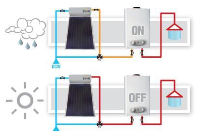
In case of insufficient irradiation and therefore the domestic hot water being modestly pre-heated, the water heater will contribute with the necessary heat to reach the required setpoint temperature.
